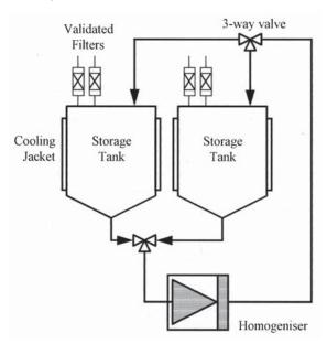
Fig. 2. Example of a high-pressure homogenization system.
